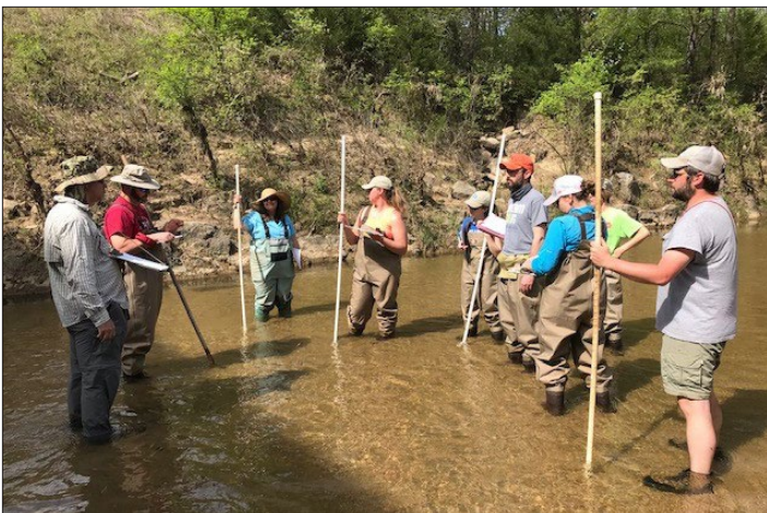
Figure 3. Performed in conjunction with a fish collection, in-stream habitat assessment involves recording data at transects every 20 meters over a 400-meter reach of the stream. Some information is based on conditions at the transect, and some is based on the full 20-meter area. Water width, water depth, substrate type, instream cover, bank erosion, and canopy are some of the recorded parameters. For this unit at Fish School, participants work both independently and in teams to complete the habitat form, which is then compared to the average score of the instructional staff.
