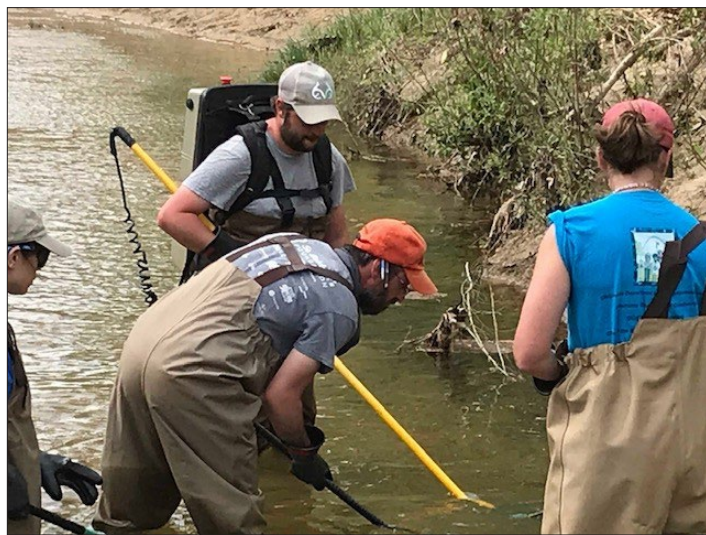
Figure 1. Using fish shocking equipment and netting the stunned fish provides an efficient way to ferret out fish in difficult locations. Both large and small fishes are stunned by the electric field for quick observation, then they are returned to their home.
