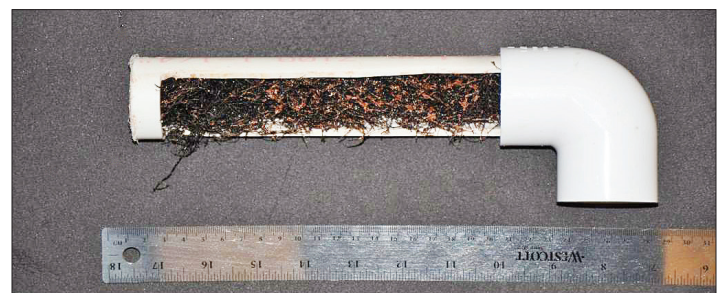
Pipe with strip inserted and elbow maintaining desired angle.
