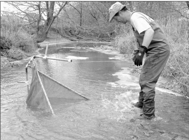
Counterclockwise from top left: Fig. 1. Handles unscrew for easy transportation. Fig. 2. Handles are positioned for running the seine or setting for a downstream kick. Fig. 3. The net can stand alone as a tripod. If the current is too strong, use the cord to hold the net in place. Fig. 4. Swivel handles to increase net's reach. Fig. 5. Left joint, front and back view.
